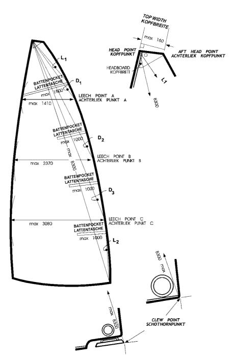
D1 - HEAD POINT TO LEECH POINT A = 2100 D2 - HEAD POINT TO LEECH POINT B = 4200
